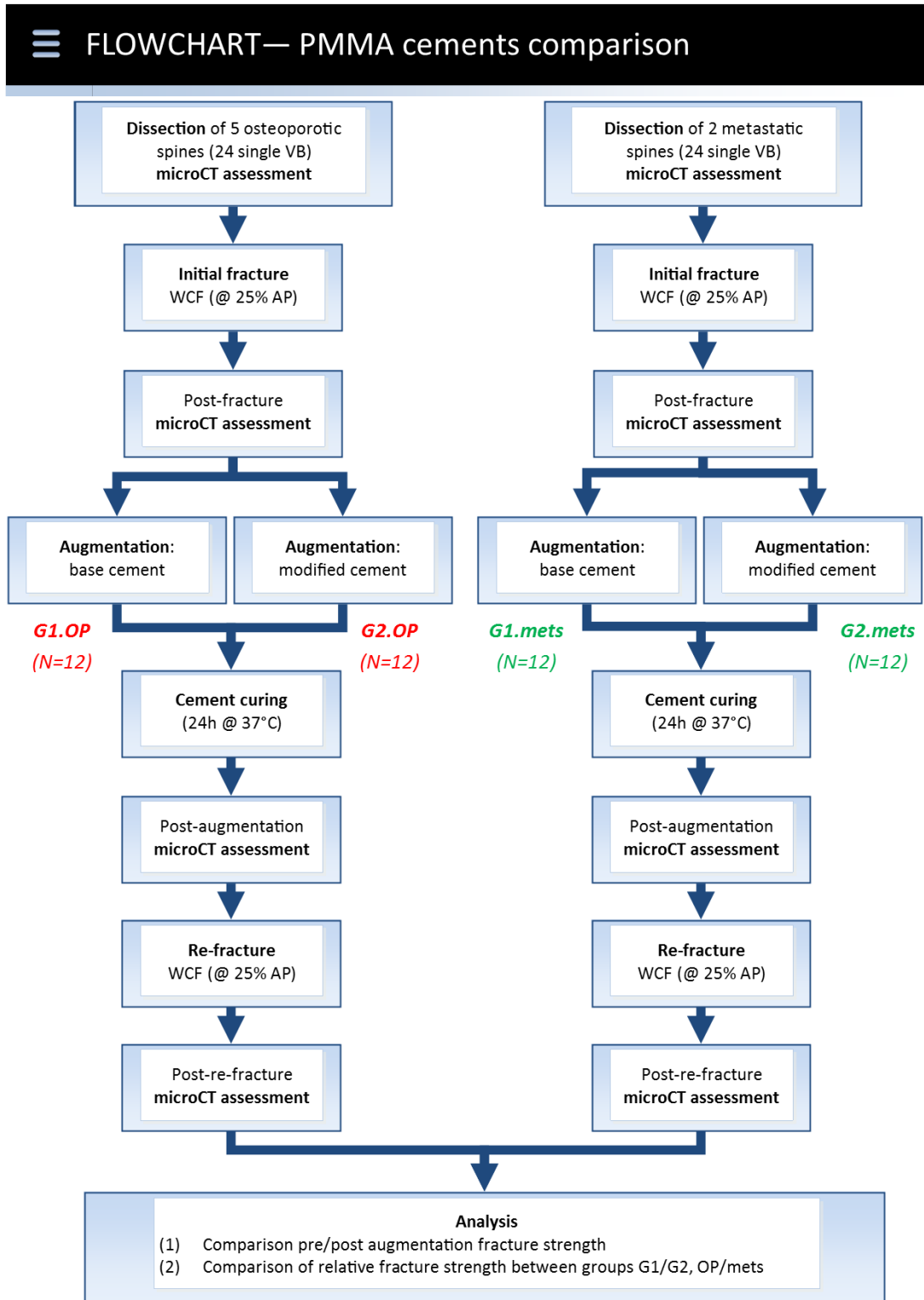
Figure 59: Study flowcharts for two scenarios, osteoporotic (a) and metastatic (b) vertebral augmentation studies comparing two cements: non-modified cement (G1) and one with enhanced formula (G2)
