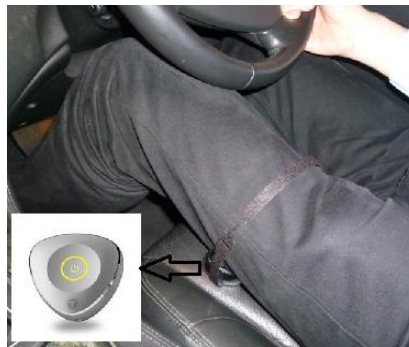
Figure 4.7: The position of the vibrating mechanism for tactile detection task during study
