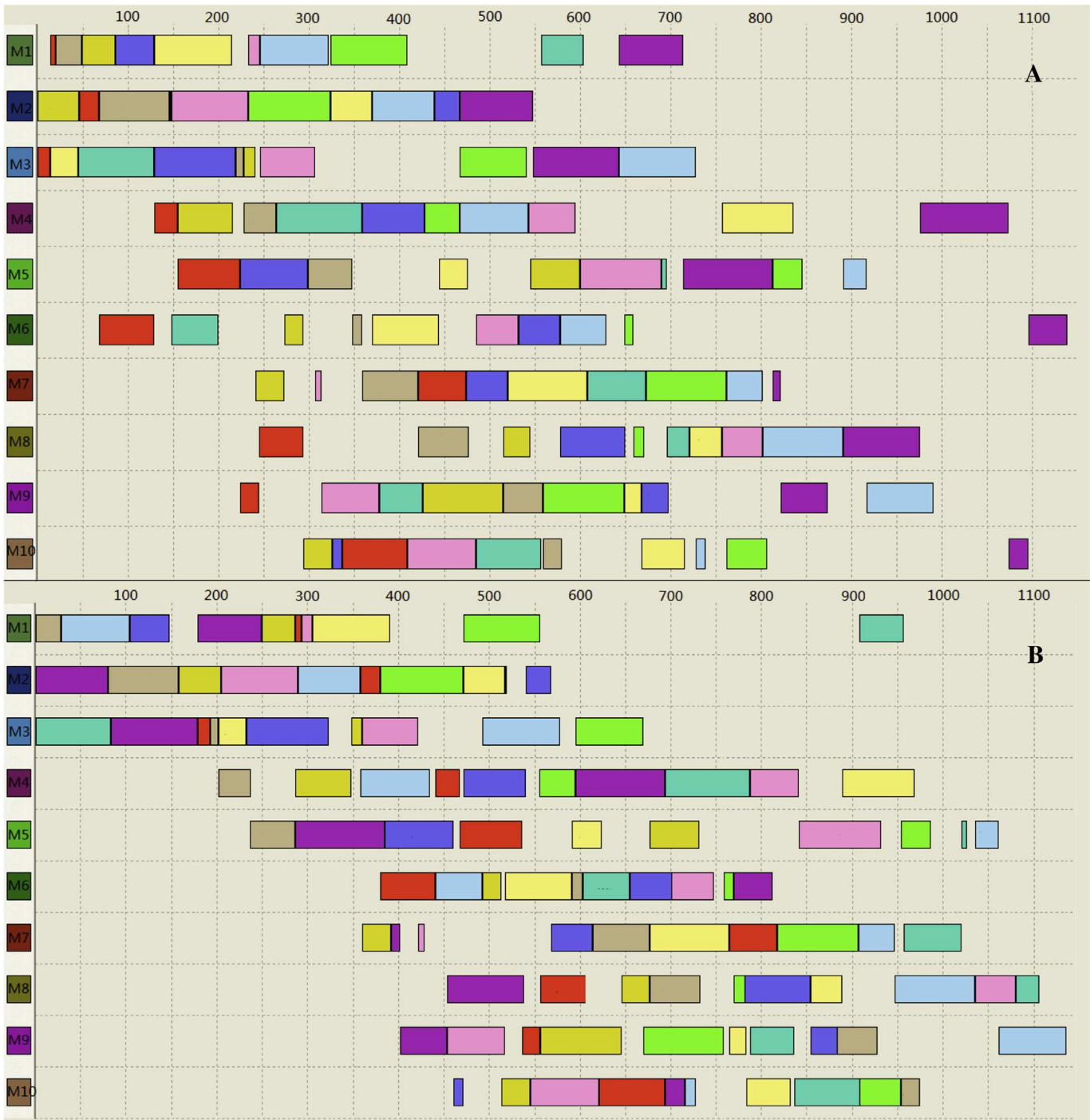
Fig. 9. Gantt chart of optimised schedule of SBH produced by LEKIN (A) and Gantt chart of optimised schedule of NSGA-II (B) while k = 1.5 .
