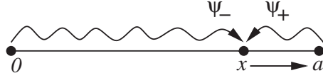
Figure 3. A schematic illustration is given of the diagonal and nondiagonal contributions to the boundary integral equation in the one-dimensional case. As the interior point x approaches the boundary point a , the off-diagonal contribution \psi_- to (2) represents a wave originating at 0 and moving towards the selected boundary point a . The diagonal contribution \psi_+ represents a wave emerging from a and moving away from the boundary.
