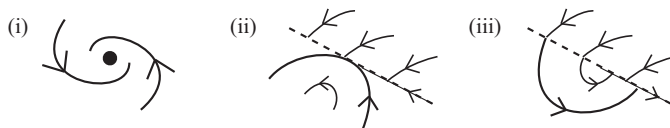
Figure 1: Simple singularities: (i) a stationary point, (ii)-(iii) tangencies between a flow and a line of discontinuity (dashed), known as (ii) a visible fold or (iii) an invisible fold.
