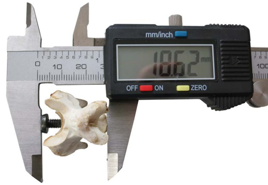
Figure 10. Modified calipers for measuring functional vertebral length. Modified calipers used to measure functional length of a turkey vertebra. The tooth glued to the left jaw protrudes into the transverse concavity of the anterior articular surface and the dorsoventral concavity of the posterior articular surface straddles the right jaw. doi:10.1371/journal.pone.0078214.g010
