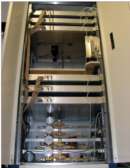
Figure 1. Frontal view of the prototype setup. The six aluminum cassettes are divided in two groups separated by a gap to insert test materials. The gas mixing system is visible on the bottom of the setup.
