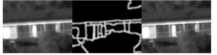
Fig. 7. Left: Region-based fusion result without the mask. Middle: Mask B^{\theta,l} . Right: Enhanced result with the mask
