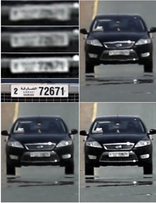
Fig. 13. Mirage sequence (B6). Top-left: Magnified number plates of (from top) original frame, SVOLA, CLEAR and undistorted frames captured at closer distance). Top-right: Original image. Bottom-left: Result of SVOLA. Bottom-right: Result of CLEAR. Again it should be noted that BD and SVOLA results use CLEAR's preprocessing.
