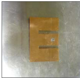
Classical metallic E-shaped antenna
