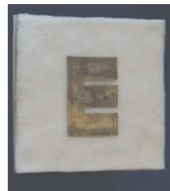
Textile E-shaped antenna with Nora
