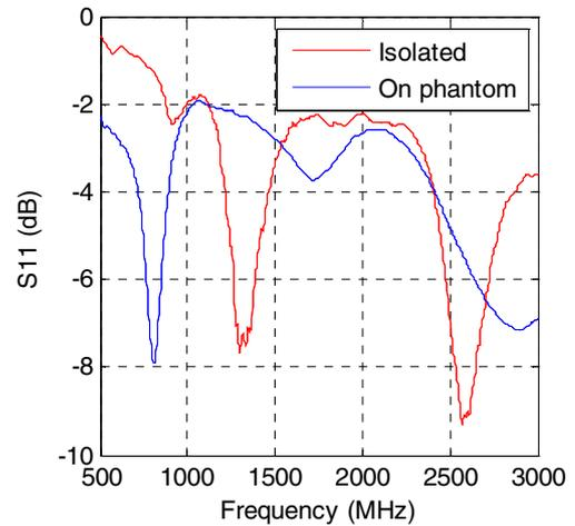
Fig. 5 Measured input response for loop antenna
