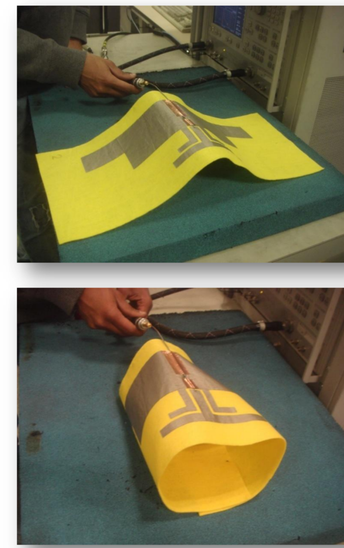
Measurements of the DTV antenna when bent or rolled showed that the input response was little affected by strong curvature
