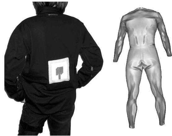
Fig. 1. Textile patch antenna on the human body. (a) Mounted textile patch antenna for a Bluetooth WPAN. (b) Curvature radii along the human body.
