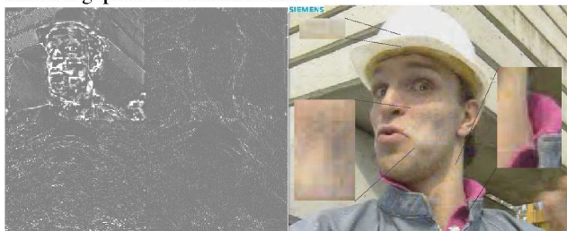
Figure 3: Highpass subbands (left) and reconstructed video (right) of frame 89 for foreman using the proposed MB-level adaptive scheme at 256kbps, refer to Figure 1 for comparison
