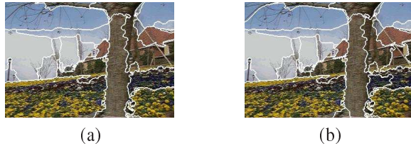
Fig. 3. Adaptive region merging results. (a) Image segmentation based on three-category. (b) Image segmentation based on two-category.
