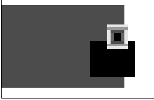
Figure 6. Sample QP map output for a frame of 'carib3'. Darker shades represent lower QP - i.e. higher quality.
