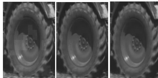
Fig. 10 Blocking effect due to FPDT (left) same frame with MRA (middle) and CPDT (right)
