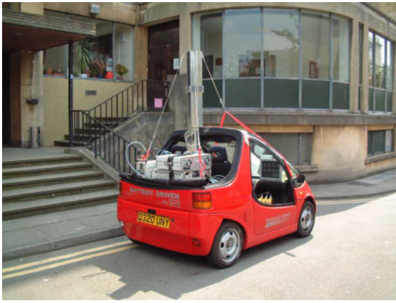
Fig. 1. ‘Mobile’ Electric Car loaded with Receiver Equipment
