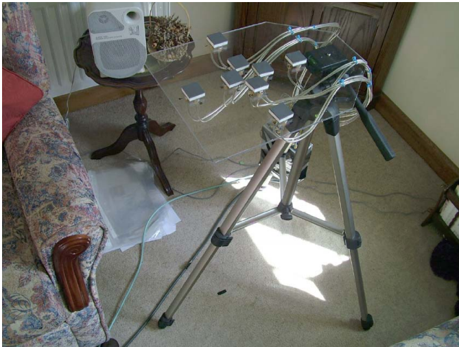
Figure 7 Rx antenna array (parallel to ground plane)
