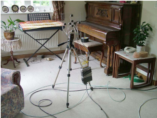
Figure 8 Rx antenna array (vertical to ground plane)
