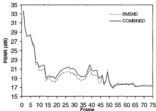
**Figure 3.** Comparison between BMSMD and COMBINED when used to conceal an H.263 encoded 24 kbits/s FOREMAN sequence corrupted with a  $10^{-3}$  bit error rate. The PSNRs are for the luminance component.
