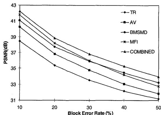
**Figure 1.** Comparison between different error concealment algorithms when applied to the FOREMAN sequence with different block error rates. The PSNRs are for whole frames and averaged over the sequence.
