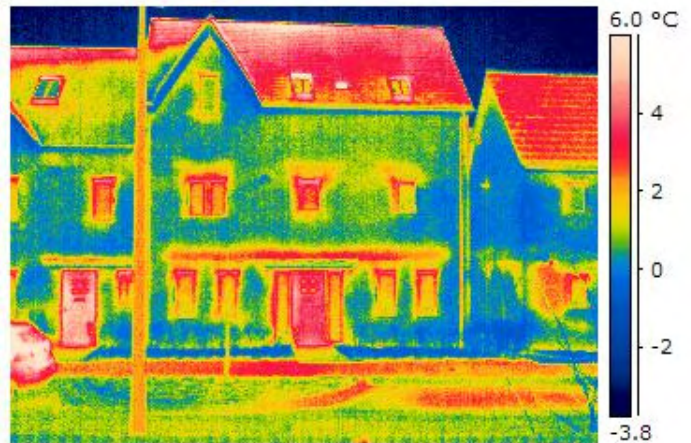
Figure 52 - Photograph and thermal image showing continuous line of thermal bridging across door and window heads in one dwelling
