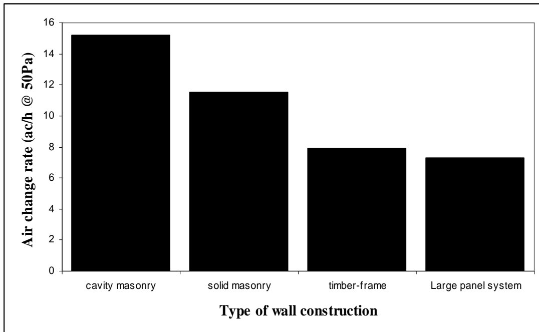
Figure 6 Influence of wall type on mean air leakage rate. After Stephen (2000).
