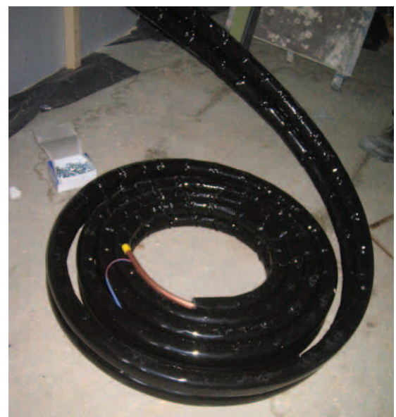
Pre-insulated malleable copper pipe used for the solar hot water system
