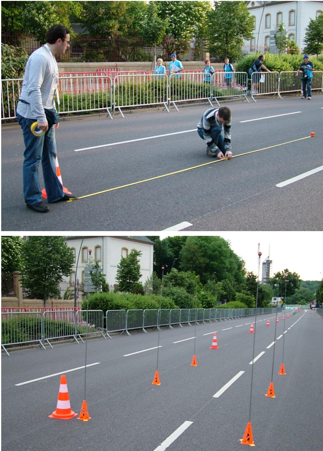
Figure 3.3. The reference volume was measured using a metal measuring tape (top photograph) and defined by six reference poles at the 8 th European Cup (bottom).
