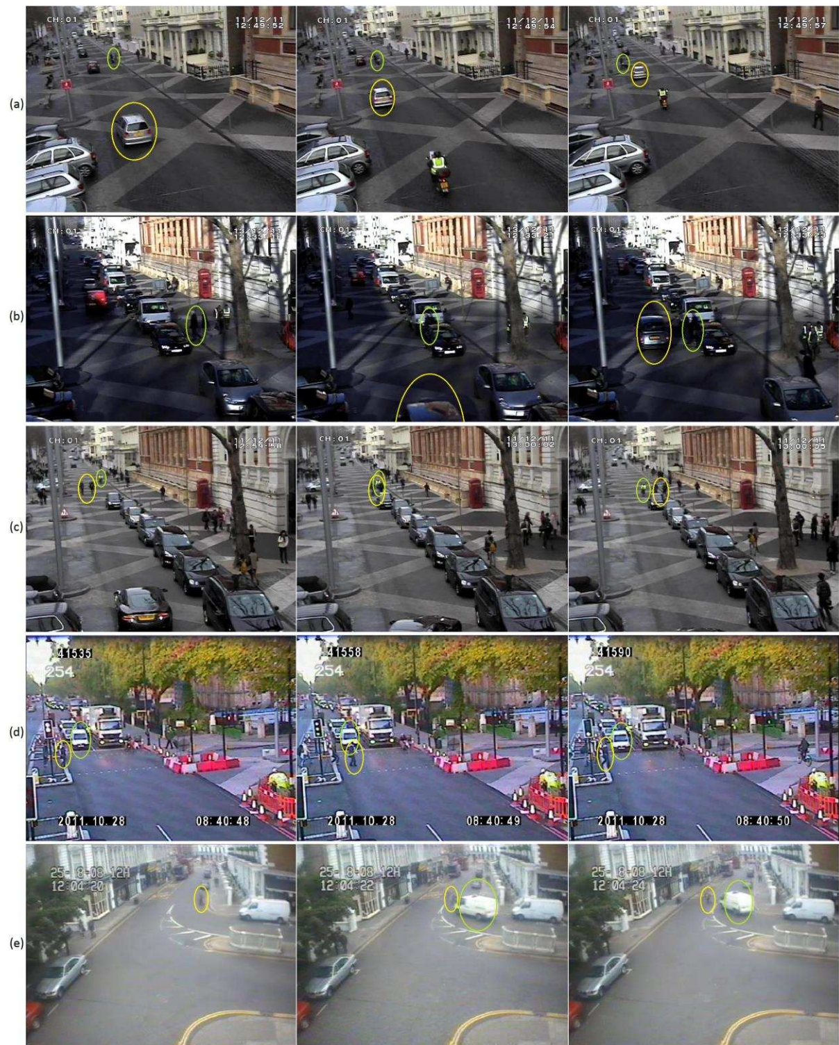
FIGURE 2: (a) Vehicle brakes in response to the crossing pedestrian, but the trajectories do not collide: No conflict (b) Pedestrians stop to let the oncoming cab pass and continue straight after: Conflict Grade 1, with factor classifications "1, 2, 1, 1"; (c) Cyclist changes course to avoid colliding with the crossing pedestrians: Conflict Grade 2, with factor classifications "2, 2, 1, 2"; (d) Pedestrian returns to pavement to avoid colliding with the departing vehicle from the stop-line: Conflict Grade 3, with factor classifications "2, 2, 3, 2"; (e) Pedestrian changes pace from 'walk' to 'sprint' to avoid a collision with the oncoming van: Conflict Grade 4, with factor classifications "3, 3, 1, 3"
