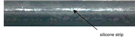
Fig. 4(b) Instrumented rebar with sensor protected by a thin layer of silicone
