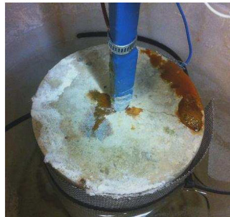
Fig. 8 Photo of corroding cylinder
