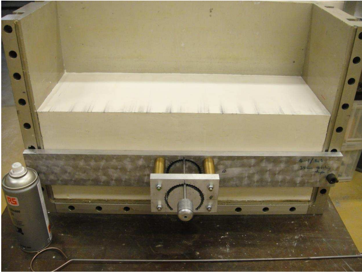
Figure 7: Forepole cavity guide and cutter
