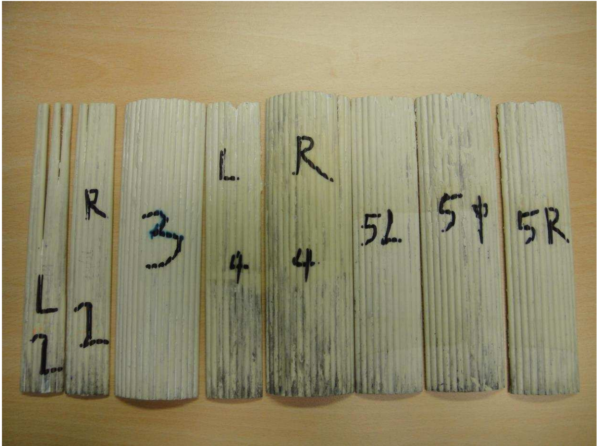
Figure 9: Quality of forepoling pouring and casting procedure (length of forpoles 200mm)
