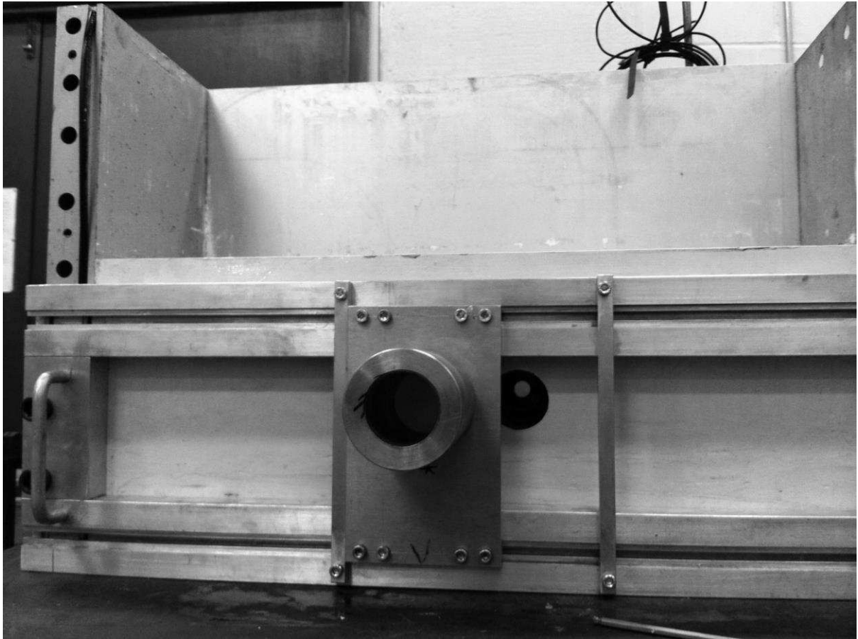
Figure 6: Adjustable tunnel cutter mounted to strong box and positioned to bore left hand tunnel. Right hand tunnel already bored
