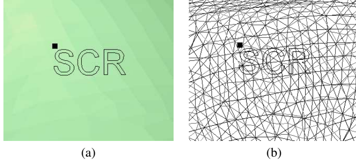
Figure 4. Positioning of the 2D text label. The user clicks the black square to drag the label into position. We show both shaded (a) and wire-frame (b) renderings.
