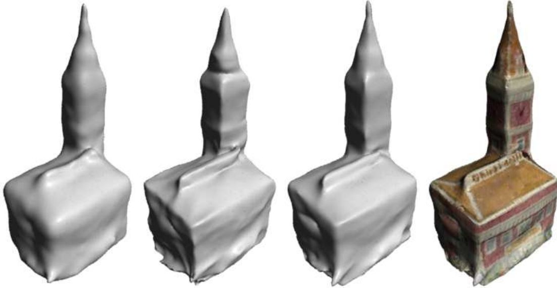
Figure 5. Comparison of reconstructions using isotropic basis (first), using anisotropic basis without additional tensor field filtering (second), using anisotropic basis with additional tensor filtering (third), and the final textured reconstruction (fourth). In all four reconstructions, \lambda = 0.001 for surface points at an edge or corner, and \lambda = 0.01 for planar points.
