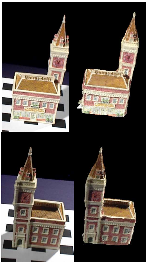
Figure 4. Actual images of the Ghirardelli souvenir model (left), and reconstructed model rendered at the same camera viewpoints (right).
