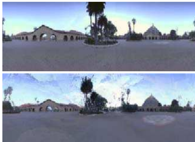
Figure 10. Above is one of ten panoramic photographs used in a reconstruction using a warped voxel space. Below is a new view rendered from the reconstruction.
