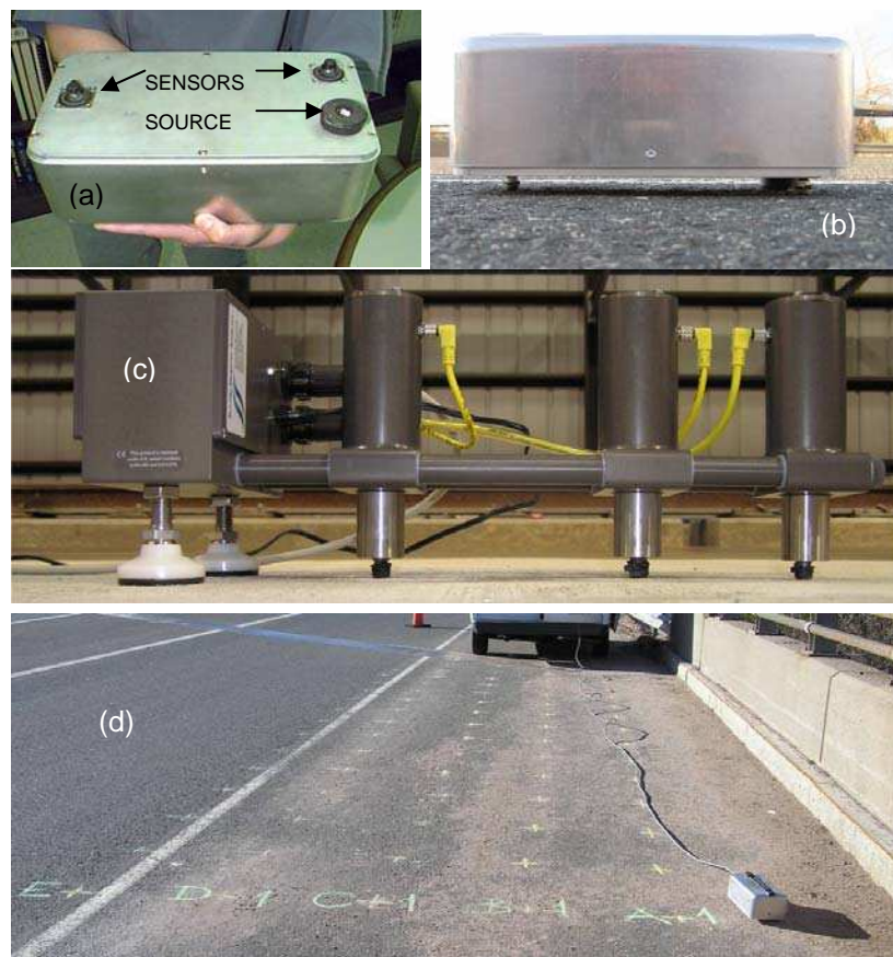
FIGURE 4 Older and newer versions of PSPA sensor box (a and c), and field implementation (b and d).
