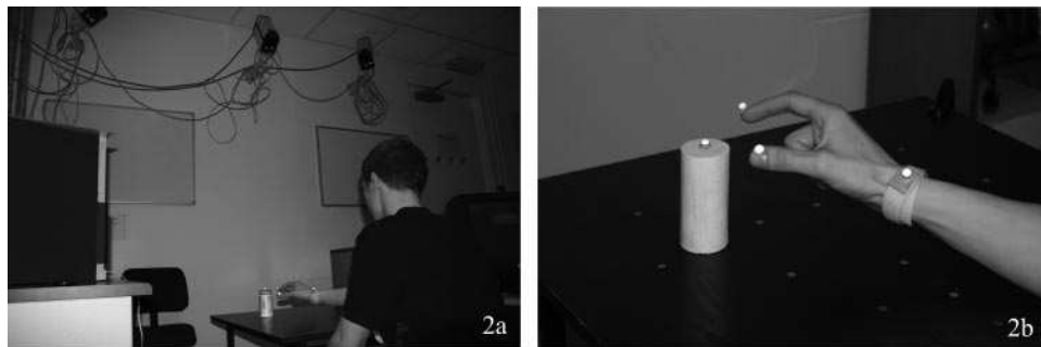
FIGURE 2. Motion capture units triangulating the workspace (a) and placement of lightweight infrared markers (b) on a subject's hand.
