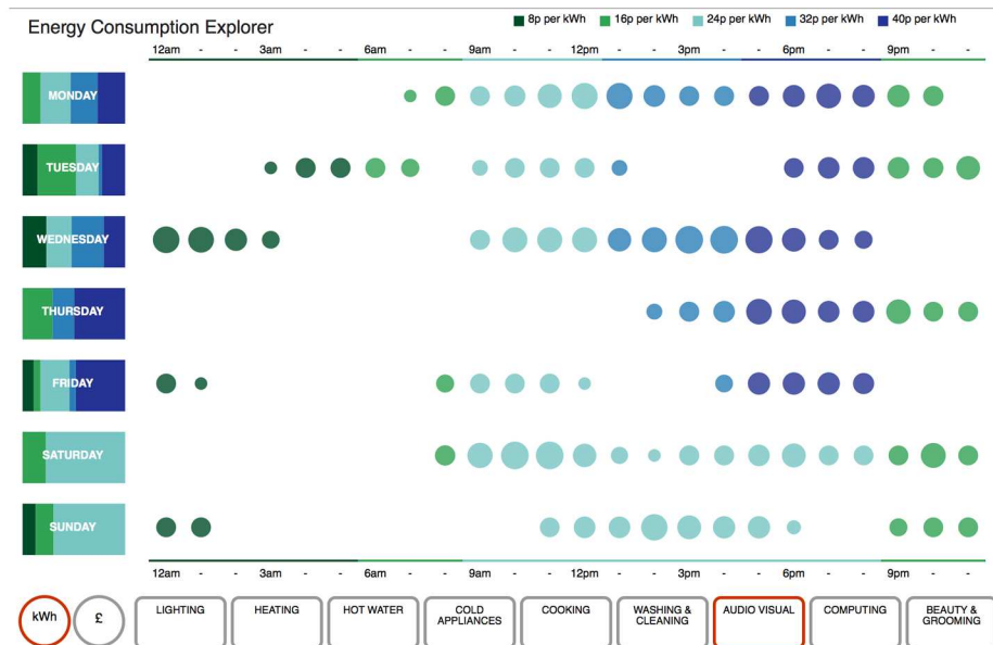
Figure 13: Screenshot of the information visualization interface filtered to show consumption of the audio visual class of appliances in kilowatt-hours
