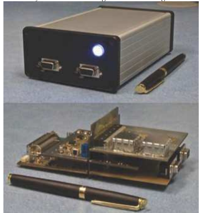
Figure 5. ZenPPG pulse oximetry processing system. The top photograph shows the front panel of the completed (all electronics are enclosed) 2-channel pulse oximetry system. The bottom photograph shows the printed circuit boards of the dual channel pulse oximetry system.
