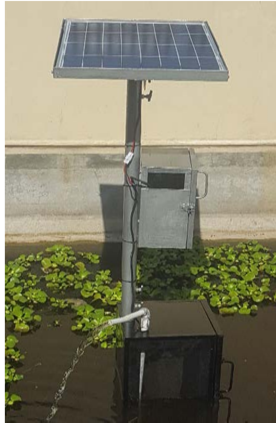
Gambar 2. Prototype pompa air portable tenaga surya
