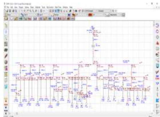
Gambar 3.3 load flow analysis ETAP Powerstation 12.6.0
