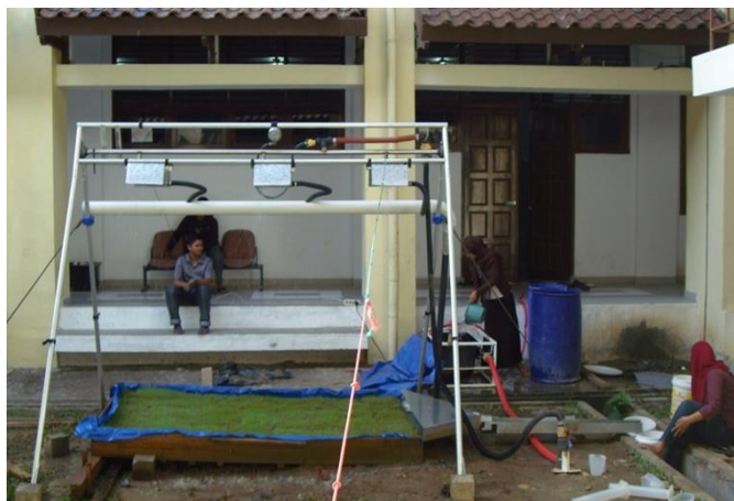
Figure 2 Rainfall Simulator and Experimental Catchment Area planted with Zoysia Japonica Grass
