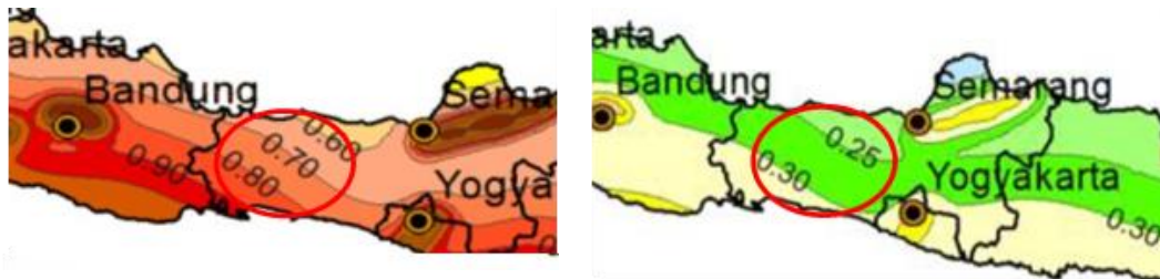
Figure 1. Spectral Acceleration response, SA, (short period, or 0.2 sec) and Spectral Acceleration, SA, (long-period or 1.0 sec) in Purbalingga regency (SNI 1726:2012)
