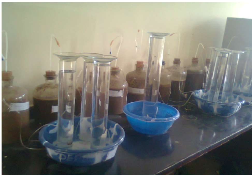
Figure 1. Diagram showing experimental setup for the biogas production
