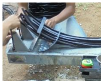
a. Tightening the waste tire on the first clamp (Maryoto, et al., 2015)
