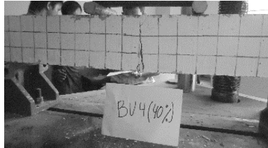
WTR-40 (Waste tire reinforced concrete with 40% tension)
