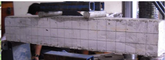
e. Setting up of concrete beam before conducting the flexural strength test
