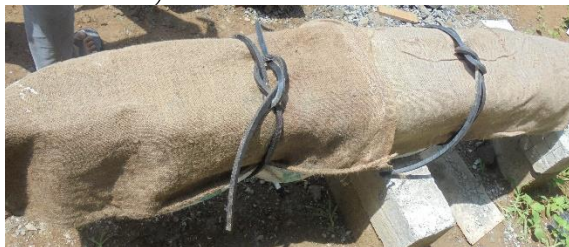
d. Curing of harden concrete specimens
