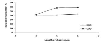
Figure 5. COD and BOD decrease by variying the length of digester
