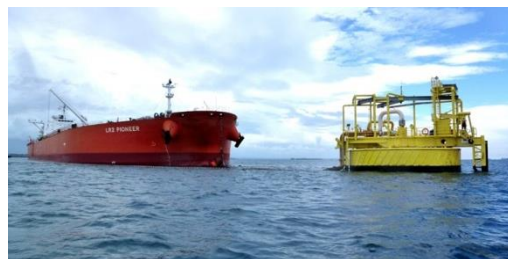
Figure 1. Single buoy mooring system [5]
