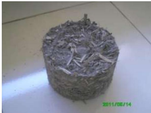
**Gambar 2.** Material agregat kasar bambu
