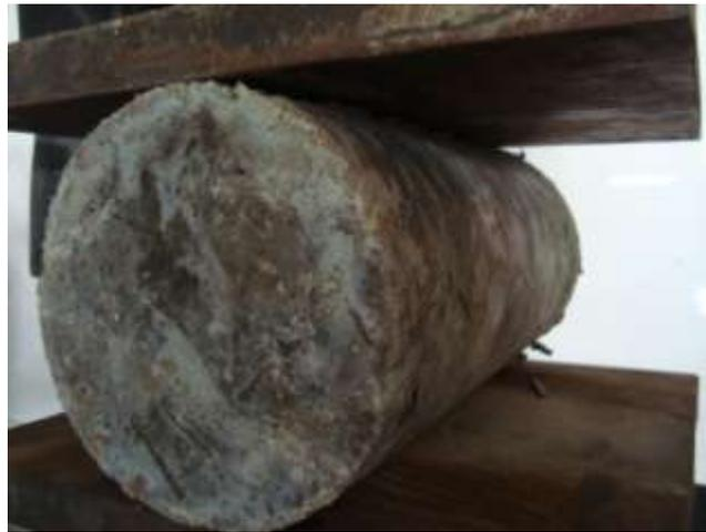
**Gambar 3.** Benda uji silinder beton-agregat bambo
