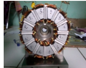
Figure 8. Stator with the winding
