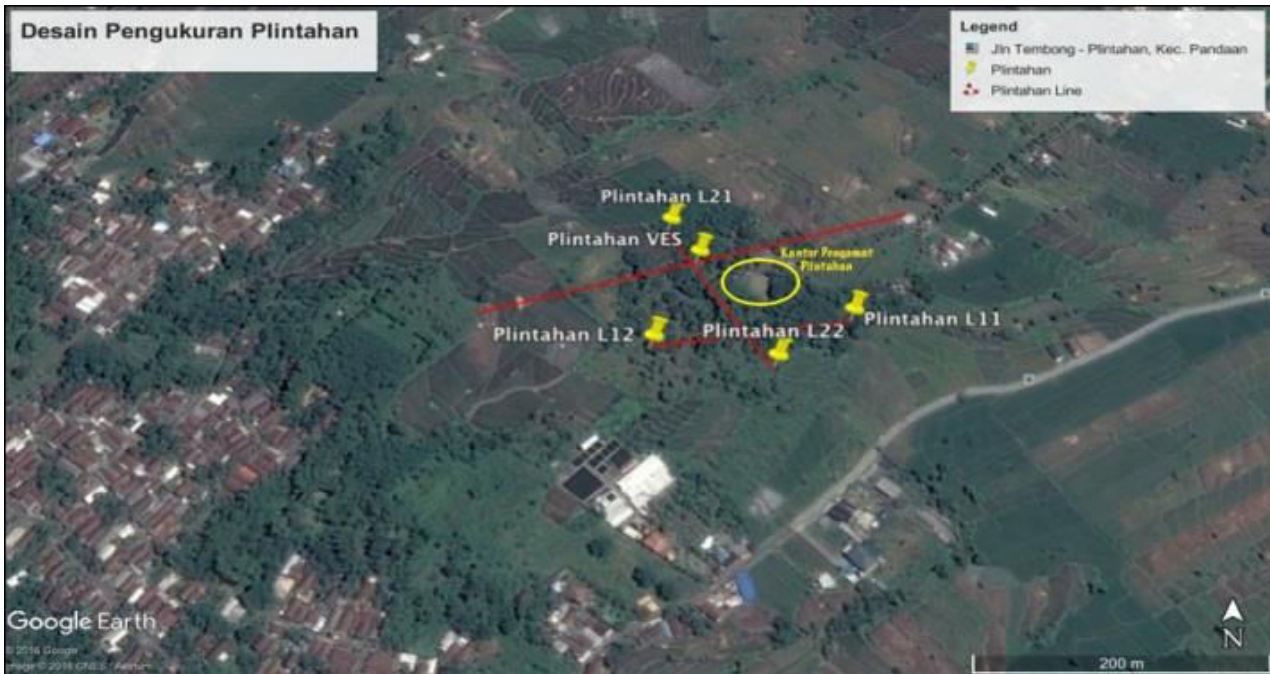
Figure 12. 2D and 1D Measurement Designs at Plintahan.
