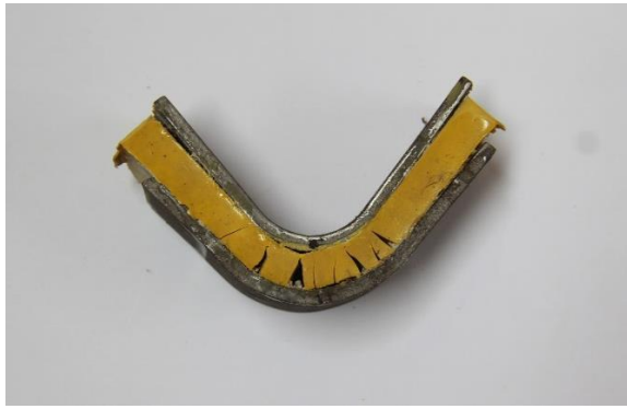
Figure 13. The last deformation of bending test.
