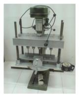
Figure 11. Gang Drilling Machine [9]
