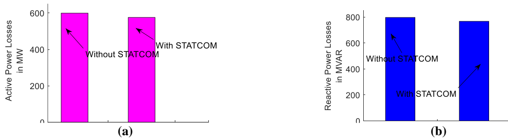
Figure 4: (a) is active power losses; (b) is reactive power losses
