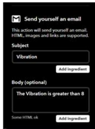
Figure 8. Screenshot for creating IFTT to set boundary limits for vibration data to send alert message
