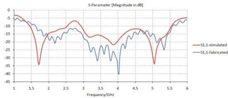
Figure 5. Simulated and measured S11 of the proposed 2x2 MIMO antenna system.
